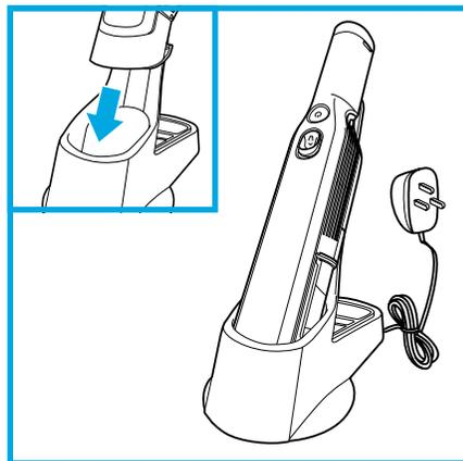
Prior to first use the lithium-ion battery must be charged completely, even if it comes with a partial charge.
