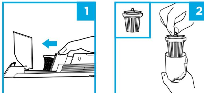
1. With the dust cup open and the power off, pinch both sides of the filter housing and slide forward to remove.
