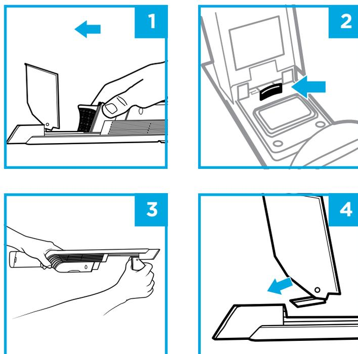
1. With the dust cup open and the power off, slide the filter housing forward to remove.
