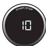
Go manual for total control of your blending speed and textures. Press MANUAL, turn the dial to select your desired speed, then press START/STOP. When selected, each speed runs continuously for 60 seconds. Press the dial again to stop the program sooner. Manual programs do not work in conjunction with the BlendSense program or Processing Mode programs.
