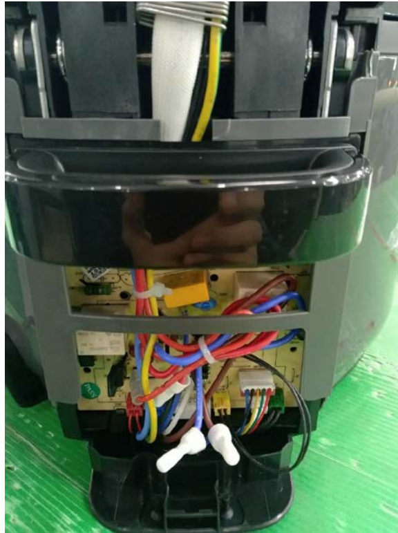
Internal view of Power PCBA position
