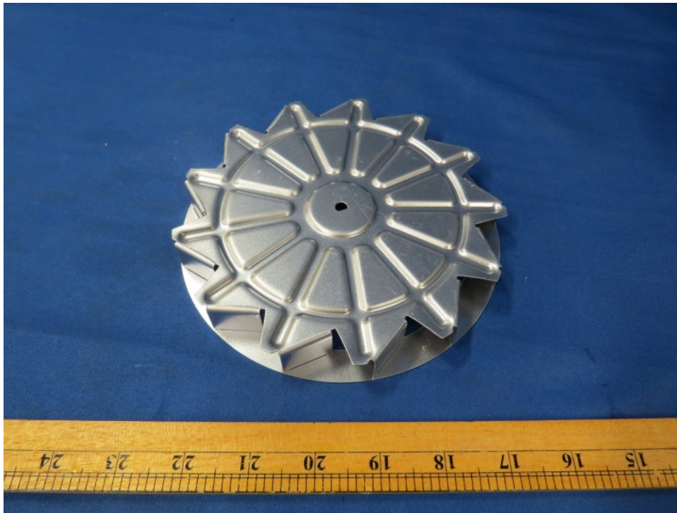
View of Air Fryer Fan Blade
