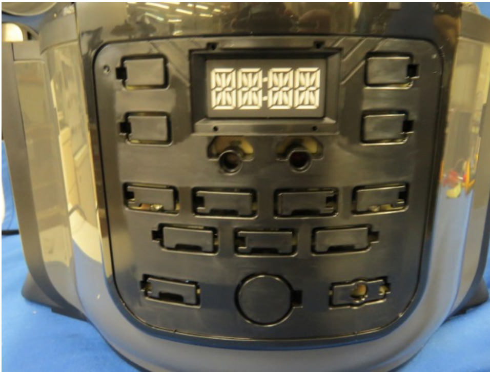
Control Panel View with UI Mylar Removed
