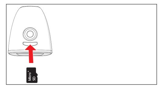
1. Insert the memory card into the Micro SD card slot.
