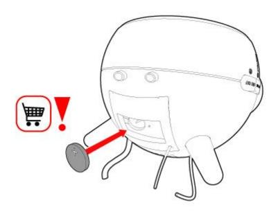
To ensure that your alarm radio remains switched on during a power outage, you can insert a battery (type CR2032). Do this as follows:
