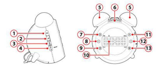
Press the (9) button . An orange bar appears in the display above AL1, the alarm is now activated. "7:00" appears on the display.
