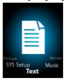
Enter TEXT mode by pressing Mode button, then you can read and edit the article in the device. The device only can recognize the article in "txt." Format.
