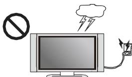
Please pull out the power plug of adapter in lightning strike, and pull out cable TV plug or outdoor antenna plug, in case the TV to be damaged.
