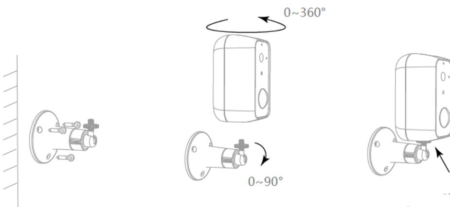
EN: Fix the bracket on the wall, install the camera in the bracket and lock it with the screw.
