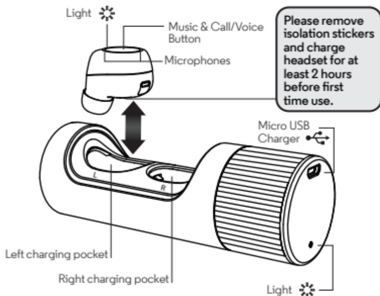
**Note:** Twist the case to open it. The case indicates which earbud is left and right. Left will be the master earbud and connect to your device, the right will automatically connect to the left.
