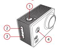
Press 2 seconds on the button OK (1) to open the menu.
