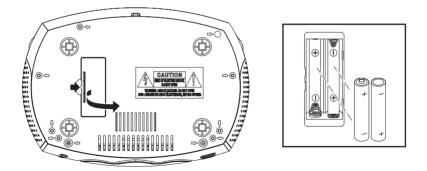
In case of a power failure, the appliance relies on battery backup. For this purpose, the appliance uses two batteries (AAA). The appliance remembers the time, but does not display it.
