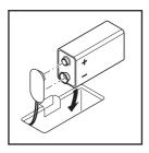
In case of a power failure, the appliance relies on battery backup. For this purpose, the appliance uses one battery (9V). The appliance remembers the time, but does not display it.
